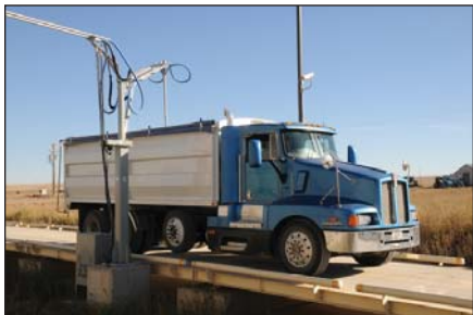
Inbound truck is weighed on a Cardinal pitless scale and sampled with an Intersystems truck probe, all under the control of a WEM automation system.
