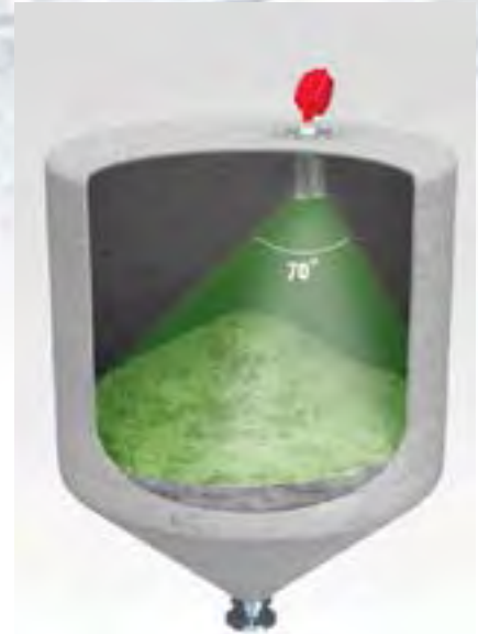
For larger silos, the M model measures multiple points within a 70° beam angle to accurately calculate volume.
