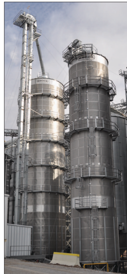
Two Brock tower dryers handle grain drying duties at Express Grain, the newer one at left rated at 10,000 bph at five points of removal and the dryer at right rated at 4,000 bph.
