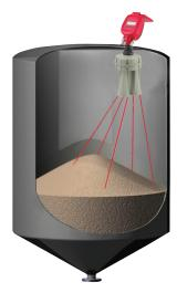
The 3DlevelScanner provides an accurate three-dimensional profile of the top surface within a storage vessel. This is beneficial when there are variations in the material surface due to multiple fill and discharge points, or with materials such as powders that do not fill/discharge symmetrically.
