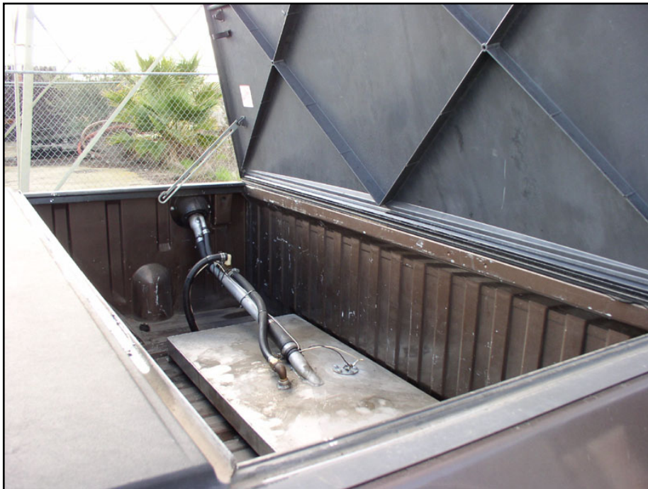
Concealed tank mounted in Division of Measurement Standards vehicle used in undercover purchases
