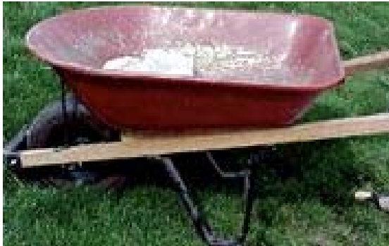
Wheelbarrow Example of Second Class Lever
