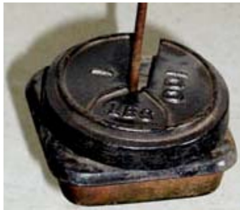
Counterpoise weight with scale ratio (1 lb. weight will balance a 100 lb. load on the scale deck)
