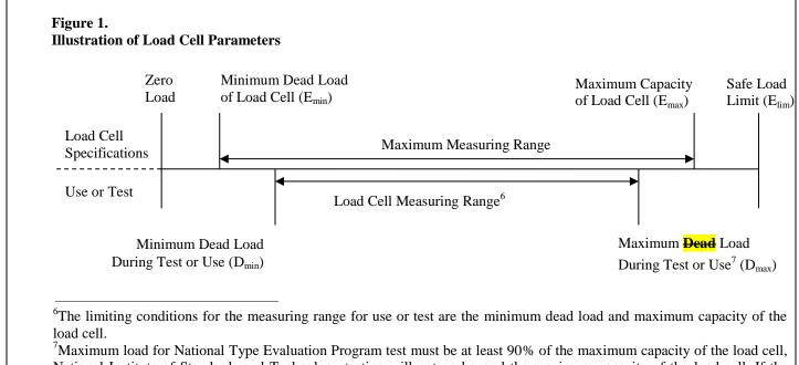
'Maximum load for National Type Evaluation Program test must be at least 90% of the maximum capacity of the load cell, National Institute of Standards and Technology testing will not go beyond the maximum capacity of the load cell. If the manufacturer test equipment limits the loads that may be applied, the manufacturer may test to a load in excess of the maximum capacity of the load cell.
